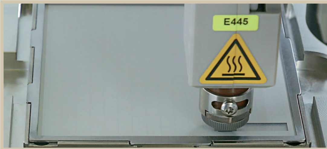
Figure 2. The pick-&-place head laminates a semiconductor die by briefly pressing it into a sinter film directly before placement
