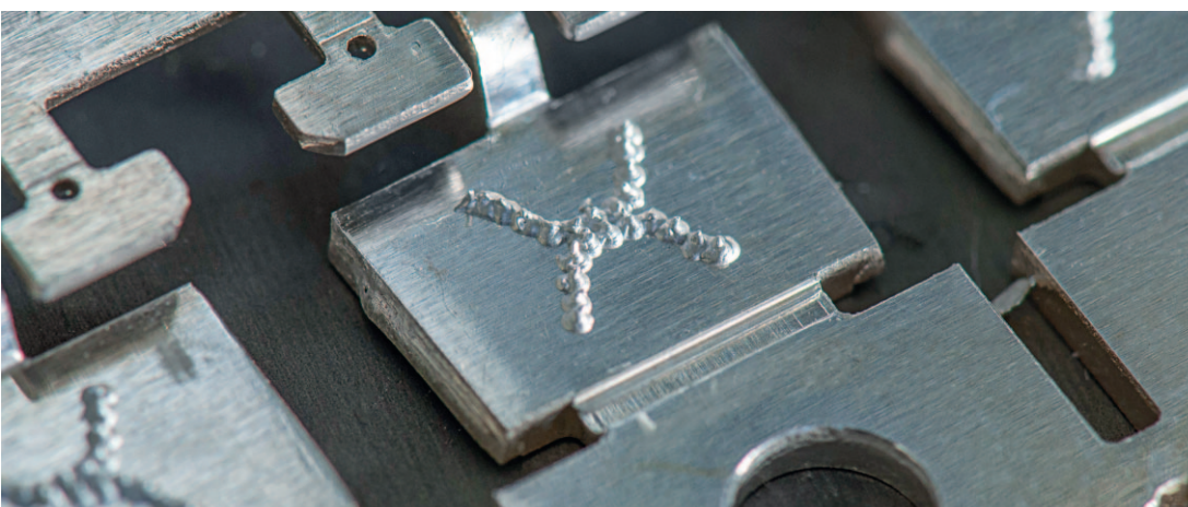
Figure 3. The sinter paste is dispensed directly onto the substrate
